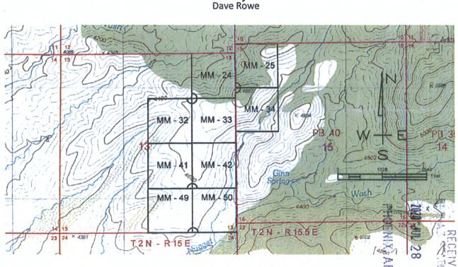
The above map depicts the \_\_\_\_\_\_MM 34 \_\_\_\_\_placer mining claim, which is located in Section(s) 15 \_\_\_\_\_\_Township \_\_\_\_\_\_North, Range 15.5 East, Gila and Salt River Baseline and Meridian, Gila County, Arizona. The claim corners and Location monuments are marked by 2 inch by 2 inch by 5 foot wooden post with atuminum tags. The bearings and distances between claims are depicted on the map.
