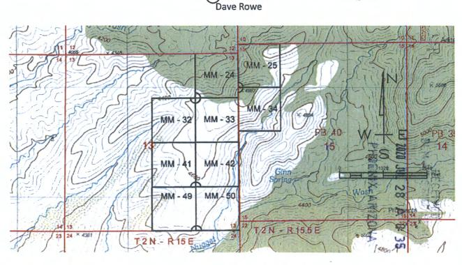
The above map depicts the MM 49 placer mining claim, which is located in Section(s) 13 Township \_\_\_\_\_ North, Range \_\_15 \_\_\_\_ East, Gila and Salt River Baseline and Meridian, Gila County, Arizona. The claim corners and Location monuments are marked by 2 inch by 2 inch by 5 foot wooden post with aluminum tags. The bearings and distances between claims are depicted on the map.
