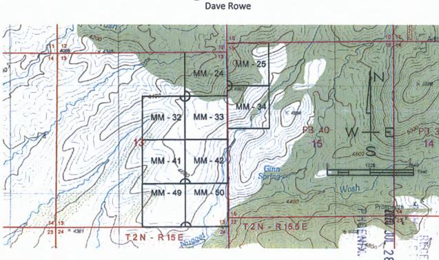
The above map depicts the \_\_\_\_\_\_MM\_33\_\_\_\_\_placer mining claim, which is located in Section(s) \_\_\_\_\_13 << Township \_\_\_\_\_2 North, Range \_\_\_\_\_5 East, Gila and Salt River Baseline and Meridian, Gila Coundy, Arizona The claim corners and Location monuments are marked by 2 inch by 2 inch by 5 foot wooden post with aluminum tags. The bearings and distances between claims are depicted on the map.
